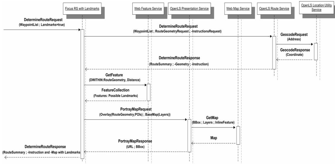
**Figure 2:** Sequence-Diagram of the Focus RS with Landmarks
