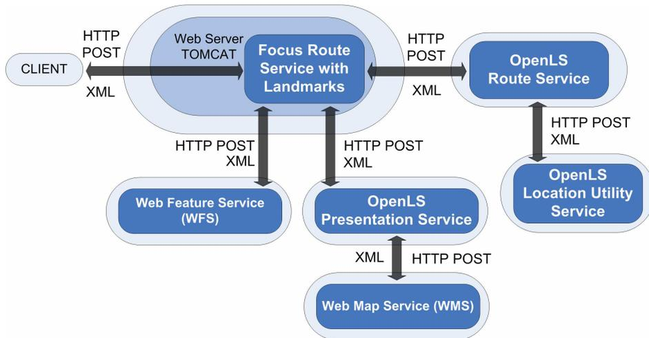
**Figure 1:** Architecture of the OpenLS Focus RS
