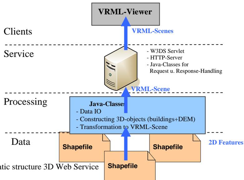
Figure Schematic structure 3D Web Service
