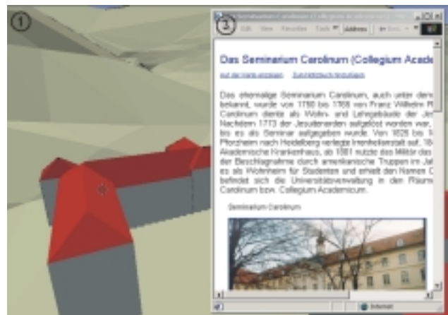
Figure 16: Using a trigger (TouchSensor) to generate a Web Page for a building from a database.
