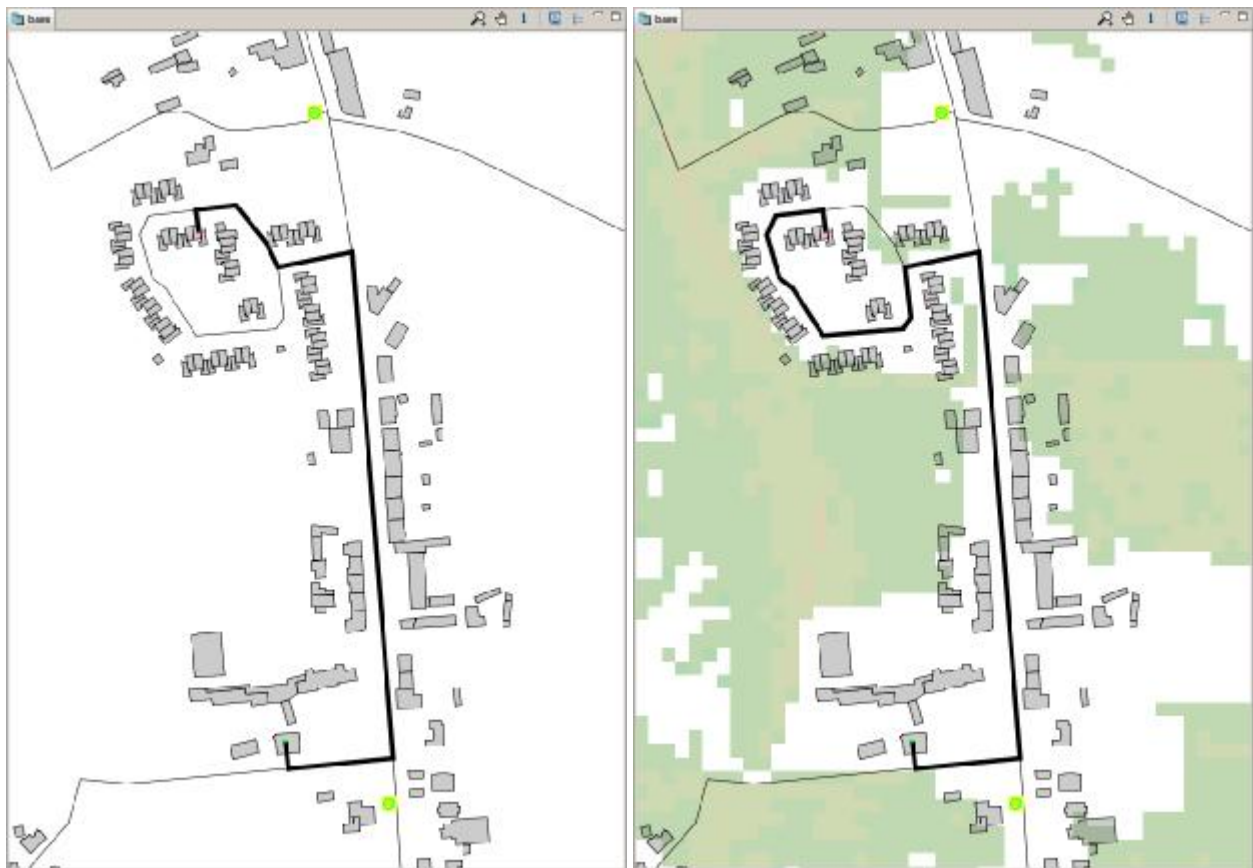
Fig. 1: Calculated routes with and without taking flooded areas into account (Kalypso User Interface)
