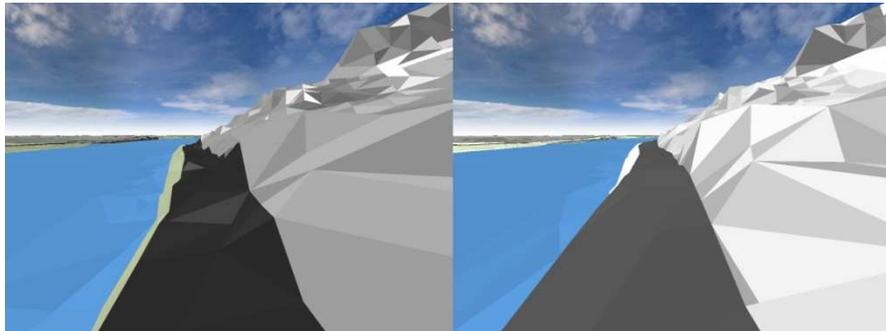
**Fig. 2: Comparison between the original terrain surface (left) and with the flattened road segment (right).**
