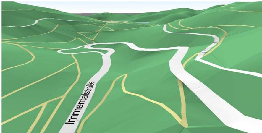
**Fig. 12: Some mountain roads integrated into the terrain and flattened. Major roads have a higher priority and have been flattened more than smaller forest tracks.**
