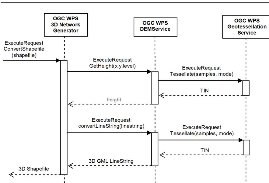
**Fig. 7: Flow chart of the 3D network generation process using OGC Web Processing Services.**
