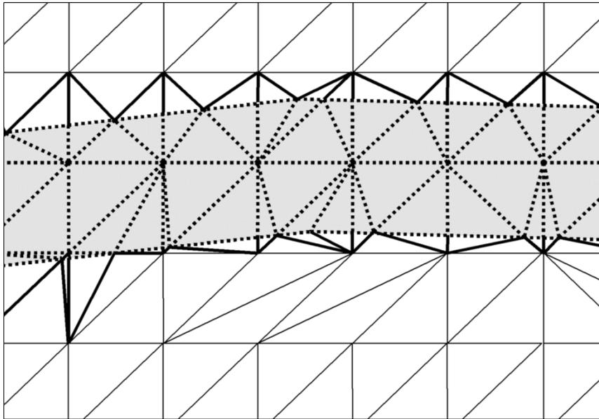
**Fig. 3: Road segment (in grey) integrated into the DTM partly modeled as spring network. During the flattening process the  $z$  value of all border and interior nodes is corrected. Length in  $R^2$  is attached to border and interior edges (dashed) as spring constant, length in  $R^3$  to exterior edges (bold).**
