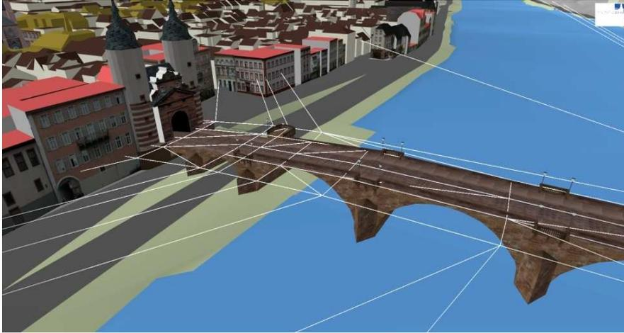
**Fig. 6:** For bridges and tunnels a second surface model is used in addition to the usual terrain (here rendered as wireframe model).
